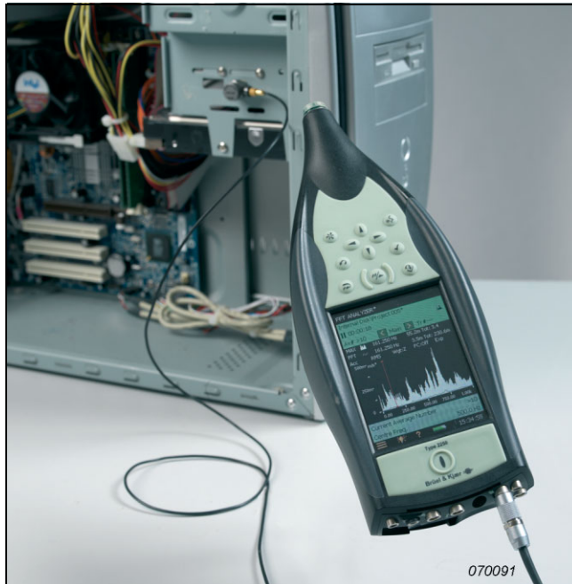
Fig. 4 Using Type 2250 for product vibration testing
