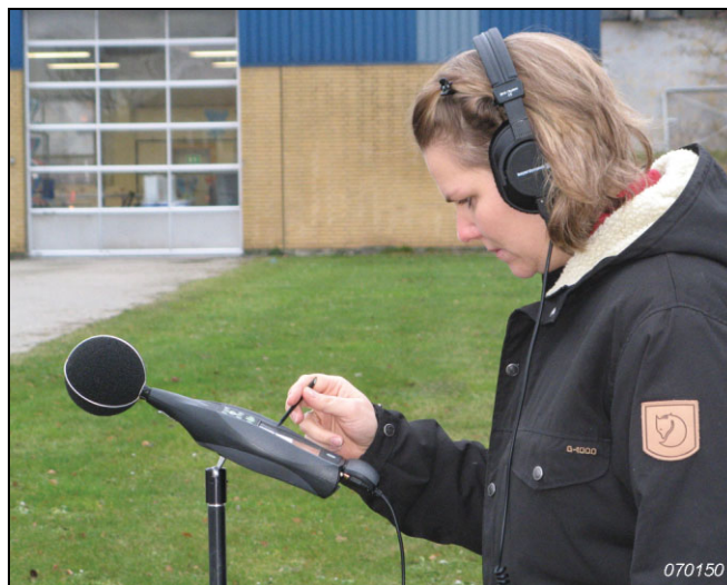
Fig. 8 Performing an outdoor tone assessment measurement
