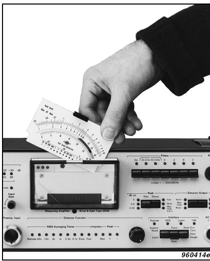
Fig.7 Insertion of interchangeable meter scale for direct reading of measured sound, vibration and voltage levels
